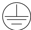
3872 – Earthing marking. The earthing marking in the drawing (connection side of the unit and the side of the unit where the terminal box is located respectively) shows the earthing point for earthing connection on site. The earthing connections on the unit itself are also marked with this label (not shown in the drawing).
